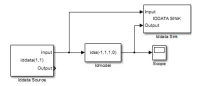
6 In the Simulink model window, connect the blocks to resembles the following figure.
