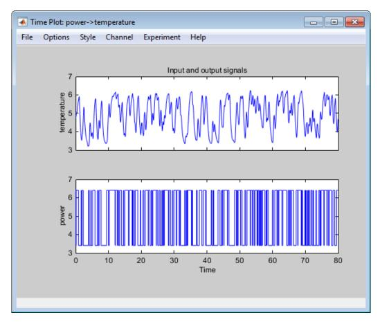
The top axes show the output data (temperature), and the bottom axes show the input data (power). Both the input and the output data have nonzero mean values.
