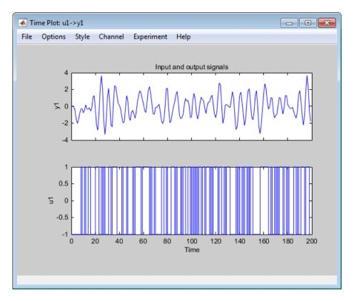
The bottom axes show the input data—a random binary sequence, and the top axes show the output data.
