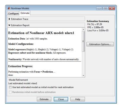
**Note Fit (%)** is computed using the estimation data set, and not the validation data set. However, the model output plot in the next step compares the fit to the validation data set.
