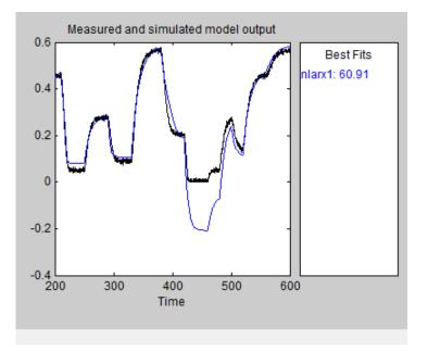
The **Best Fits** area of the Model Output plot shows that the agreement between the model output and the validation-data output.
