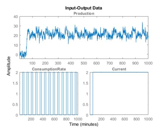
Zoom in on the plots to see that the experiment process amplifies the first input ( ConsumptionRate ) by a factor of 2, and amplifies the second input (Current ) by a factor of 10.
