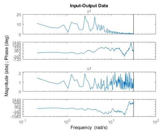
• **Frequency-response data** — Specify as an idfrd object. If you have Control System Toolbox software, you can also specify the data as an frd object.
