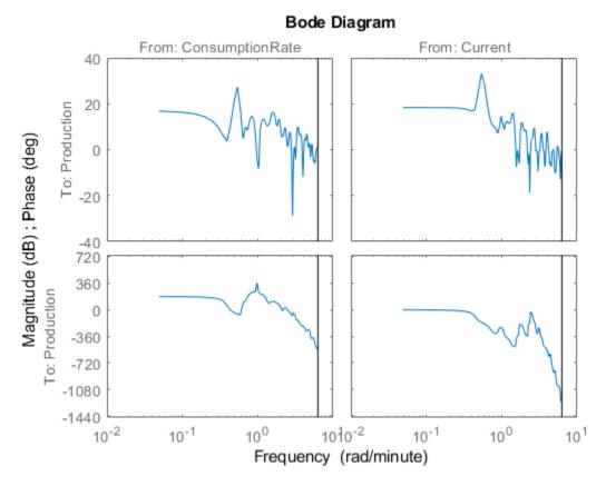
The amplitude peaks at the frequency of 0.54 rad/min, which suggests a possible resonant behavior (complex poles) for the first input-to-output combination - ConsumptionRate to Production .
