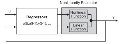
The software computes the nonlinear ARX model output *y* in two stages:
